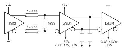
Figure 14. Interfacing from LVDS to Negative Supplied ECL
