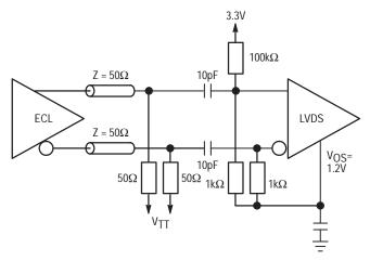
Figure 6. Capacitive Coupling ECL to LVDS Using VOS
