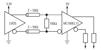
Figure 12. Interfacing from LVDS to PECL
