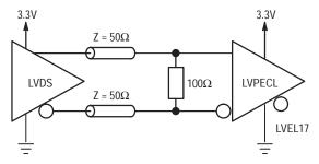
Figure 9. Interfacing LVDS to LVPECL
