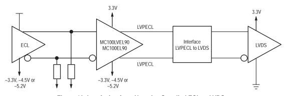
Figure 13. Interfacing from Negative Supplied ECL to LVDS
