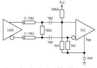
Figure 3. Capacitive Coupling LVDS to ECL Using VBB Several ECLinPS/ECLinPS Lite devices supply a VBB (VBB  $\approx$  VCC-1.3V) reference voltage. It can been used for
