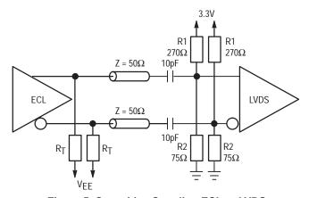
Figure 5. Capacitive Coupling ECL to LVDS
